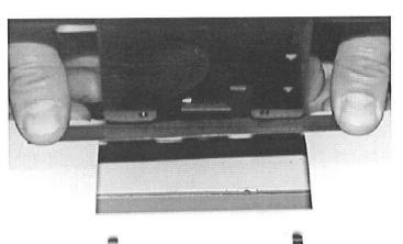
Step 4. Remove the insert suction cup. Lower and tilt the adjustable sucker assembly forward. Plug the sucker hose. The sucker assembly may be moved down and to one side if it interferes with the material being fed.
