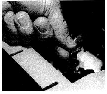
Step 4. Remove the insert suction cup. Lower and tilt the adjustable sucker assembly forward. Plug the sucker hose. The sucker assembly may be moved down and to one side if it interferes with the material being fed.
