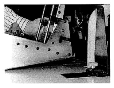
Step 7. Place the feeder on the rear insert table with the two screws that protrude from the bottom of the feeder aligned into the rear guide slots. Secure the feeder with the two "T" Handle nuts provided.
