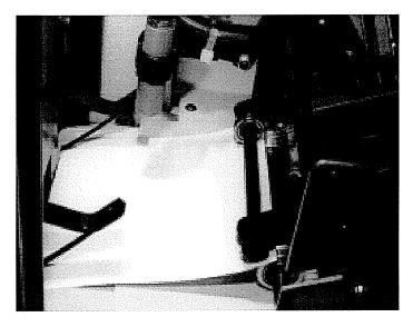
Step 8. Feeder positioning. Place a piece of material to be run under the spring steel guides. Have the front edge of the material aligned with the front of the insert plate. Slide the feeder toward the gripper arm until the trailing edge of the material held by the guides fits between the feeder's exit rollers.
