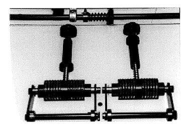
CAUTION: Before running the feeder, be sure that the gate cylinder is adjusted upwards enough that the "O"-rings are not contacting the feed rollers and belts. If the gate cylinder "O"-rings are in contact with the belts and rollers and the feeder is run with no material in it, you will damage the belts, rollers and "O"-rings.
