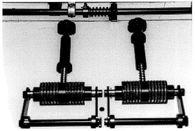
The "O"-rings are worn to the same height as the gate cylinder. Turn or replace all "O"-rings if they are worn.
