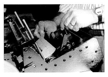
Step 11. Material Support Wedge Adjustment. The trailing edge of the material to be run *must* be supported by the material support wedges.
