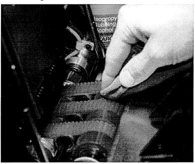
Clean rollers and belts are VERY IMPORTANT to the proper operation and feeding of the Streamfeeder!
